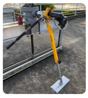
**U.S.SAWS** Valve Exerciser - Treatment Plant Application (US75060) is a powerful, lightweight, battery-operated unit designed to take away from labor-intensive hand-cranking motion in a water reclamation plant.
