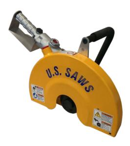
The U.S.SAWS hand-held, air-powered saws are an alternative to traditional gas-powered chop saws. Air-power is more reliable, longer-lasting, and emits no hazardous exhaust fumes. Ideal applications are confined space cutting, underground applications, or operation in interior space.
