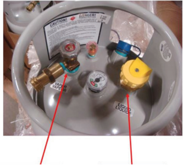
Propane Service Valve on Vapor Port
