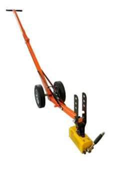
U.S.SAWS Supreme Duty Collapsible Dolly Manhole Lifter is a versatile tool with the power to get the heavy lifting while avoiding back injuries associated with lifting maintenance hole covers. The unit is compact and lightweight, allowing it to fold down for easy storage and shipping. The dolly eliminates the use of pry bars, ensuring user safety, and moves covers up to 36".
