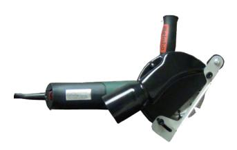
The U.S.SAWS 5" Crack chaser is a hand-held crack chasing saw designed to rout out random cracks before filling. This saw is also used for cutting repair patches in concrete surfaces where a dust-free environment is needed. It can also be used for joint clean-out and joint fill removal in areas where the larger joint clean-out saws will not fit. The full metal blade guard protects the operator, and the dust shroud is durable enough to hold up to abrasive concrete dust.
