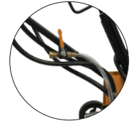
WATER FEED HOOK UP
