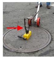
Moving the lifting pin on the magnet (three positions available) alters the height of the trolley handle. This allows the user to select an operating position that best suits their height or stature.
