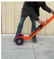
Pull the stray bar connector and then fold the bottom arm up to the middle
