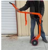
Push the side button in the middle of the dolly down and then push the top handle down
