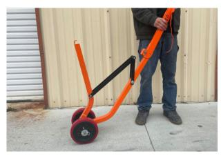
Straighten until the stray bar connector snaps into place
