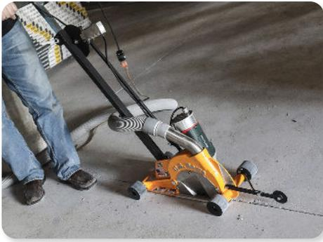
U.S.SAWS milling machine line is designed to clean- out joints and remove existing joint filler faster and more accurately. The MC-45 is great for cutting out spalled joints and other applications where concrete needs to be removed. The Mark-III is ideal for applications where joints need to be cleaned out. Both saws are designed with a heavy-duty frame providing the user with long longevity. Ease of use, high accuracy and durability are key components to U.S.SAWS line of milling machines.
