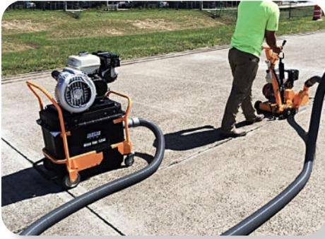
U.S.SAWS offers a wide range of joint clean-out saws to serve the concrete industrial flooring professional. The saws are designed to clean-out existing control joints and remove old joint fill material that needs to be replaced. U.S.SAWS offers the saws in a propane and gas powered option depending on the job-site and needs of the end user. Durability, accuracy and high production rates are key components to our industry leading line of joint clean-out saws.
