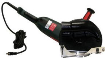
The hand-held Cut-Vac is designed for routing out cracks or cut concrete up to 1-1/8" deep while collecting the dust. The saw is also available as a stand-up unit that makes cutting straight decorative cuts or cleaning out control joints faster and easier.
