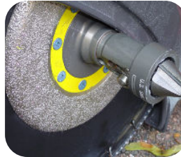
Ductile Iron and PVC Beveller installed on Chop Saw with Blade
