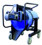
The M-22 4 Bag Mixing Station is a compact, robust mixing station with good balance when pouring the self levelling compound, even with larger mixing volumes. The mixer unit is built with a 2-speed gearbox and infinitely variable speed setting allowing for quality control and mixing power. The M-22 is compactible with cement self-levelling and materials with good liquidity.
