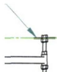
Figure 7 - Alignment of blade and the pointer wheels - JS bottom view
