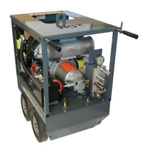
The M300 Merit hydraulic power pack is built for the professional cutter that runs all day and demands a reliable, cool running hydraulic power source. The 23-hp Kohler engine delivers power to the hydraulic pump with a variable flow control.
