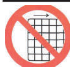
Figure 8 - Warning label - do not operate with guard removed
